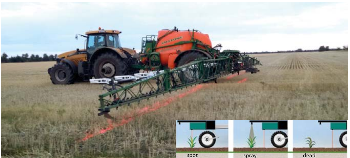
Figure 1.5: Spreader UX 5000 with the weed detection system Amaspot. The scheme shows the Amaspot system: an infrared sensor detects green/ growing weed and initiates, and stops spraying when passing over the field, in the Kulunda steppe, Russia. (photo: Lars Grunwald; illustration: Amazon-Werke)
