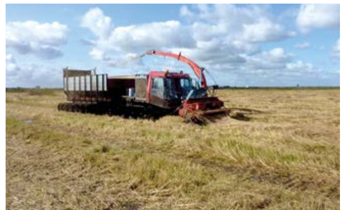
Figure 3.8: Prototype harvester for re-wetted areas. In order to retain some production from the wetlands part of the biomass is removed. (Wendelin Wichtmann)
